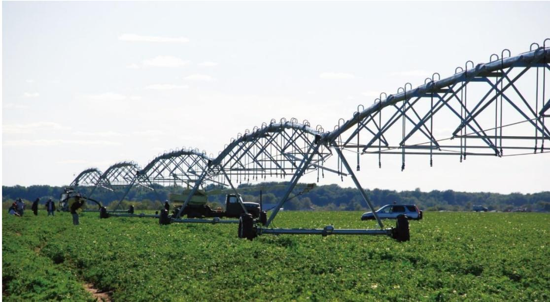
Rainfine 500 meters towable pivot in Kazakhstan is used in 3 different fields and is designed to tow every one or two weeks in 400mm high potato fields . After 4 years working, the structures and truss rods have no any distortion
