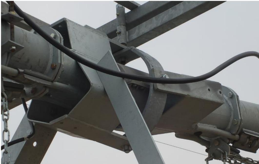
This hard but flexible joint design can support all the strength of the pivot and maximum the flexibility of the pivot joint in case that the pivot system can walk properly in waving land.
