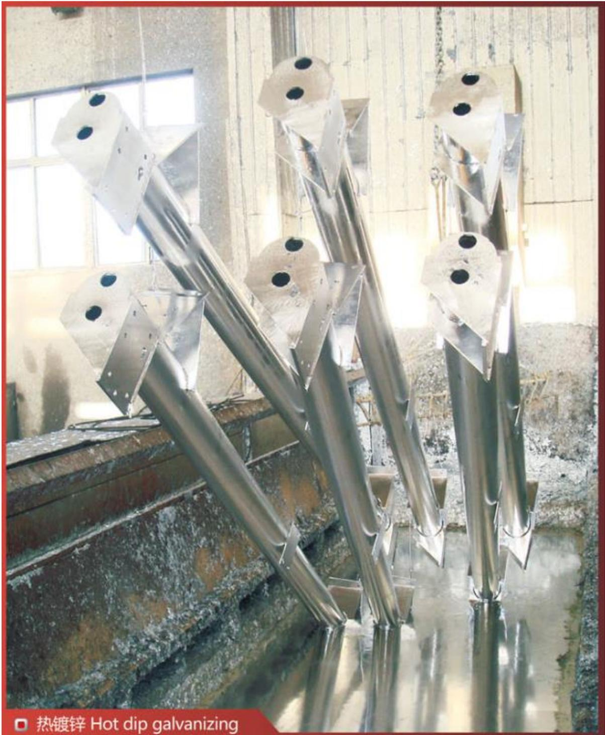
**Hot dip galvanized structures with 141 / 168 / 203mm diameters:**
