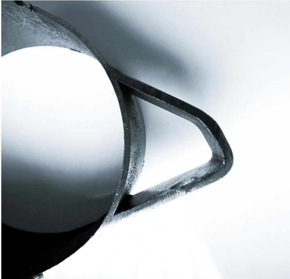
Cut the pipe from other side and see the penetration deep. It should be more than 1 mm deep. This test is done each among 200 pipes.
